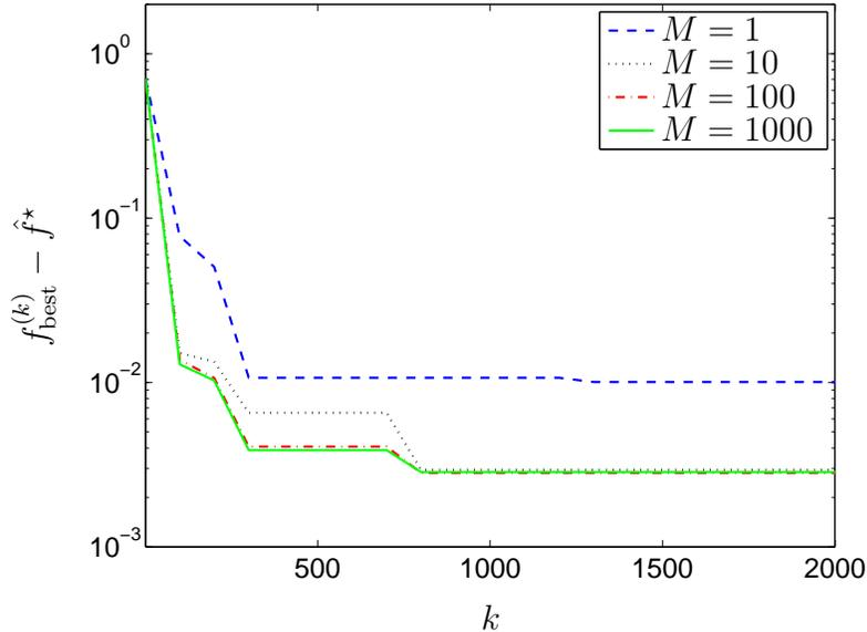
**Figure 5:** The value of  $f_{\text{best}}^{(k)} - f^*$  versus iteration number  $k$ , for the stochastic subgradient method with step size rule  $\alpha_k = 1/k$ . The plot shows one realization for noisy subgradients evaluated using  $M = 1$ ,  $M = 10$ ,  $M = 100$ , and  $M = 1000$ .
