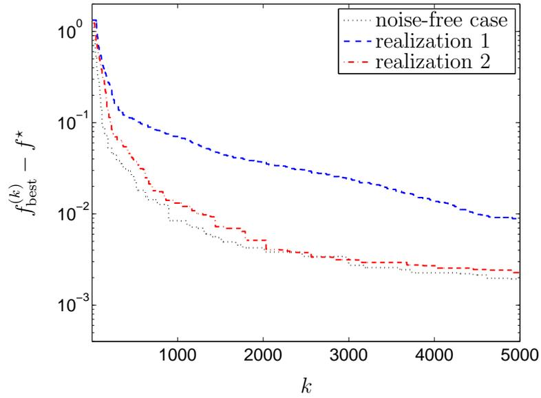
**Figure 1:** The value of  $f_{\text{best}}^{(k)} - f^*$  versus iteration number  $k$ , for the subgradient method with step size  $\alpha_k = 1/k$ . The plot shows a noise-free realization, and two realizations with subgradient noise.
